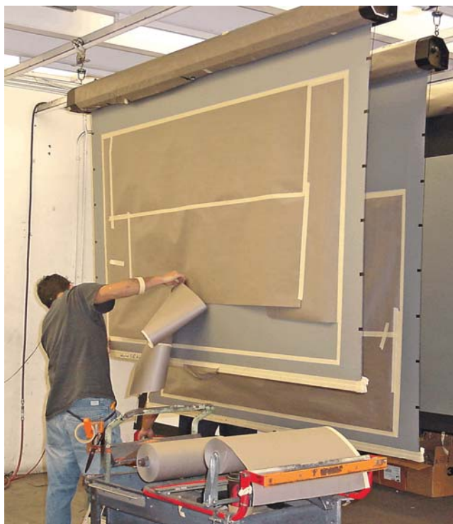
Viewing Areas of Screens Are Taped Off for Painting
