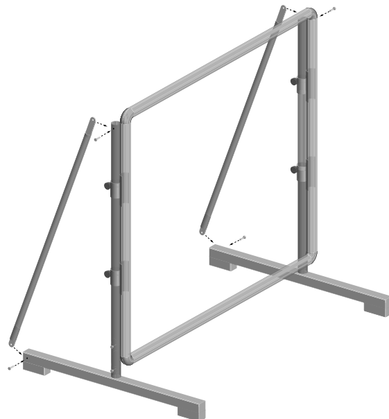
Figure 8. Attaching cross braces
