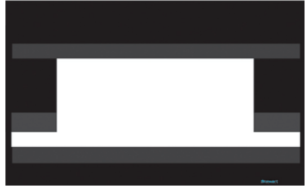
Horizontal panels drop down and rise up, while vertical panels drop down on either side to attain the desired aspect ratio.
