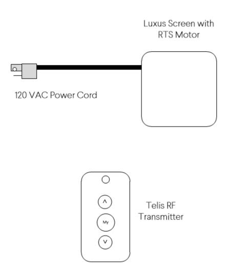
The optional Luxus RTS Motor uses a standard 120 VAC power cord. An integral RF receiver, and a dedicated hand held remote, operate the screen. The power cord plugs into a continuously powered AC outlet. With the addition of the Somfy MyLink device, the system becomes wi-fi discoverable and will facilitate control of the screen surface via tablets, phones and more.
