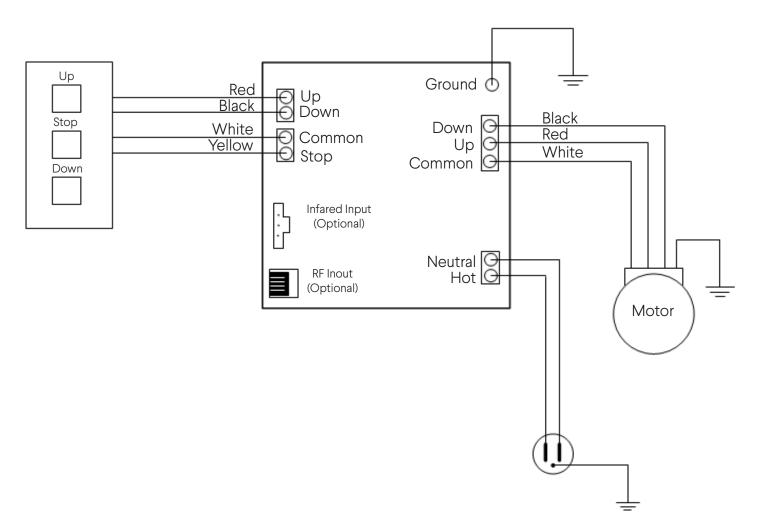
The Low Voltage Control (with Wall Switch) is a screen control that allows for switching conductors to be run in Class II (small wire, exposed, no conduit) and will interface with most outboard video switching systems.
