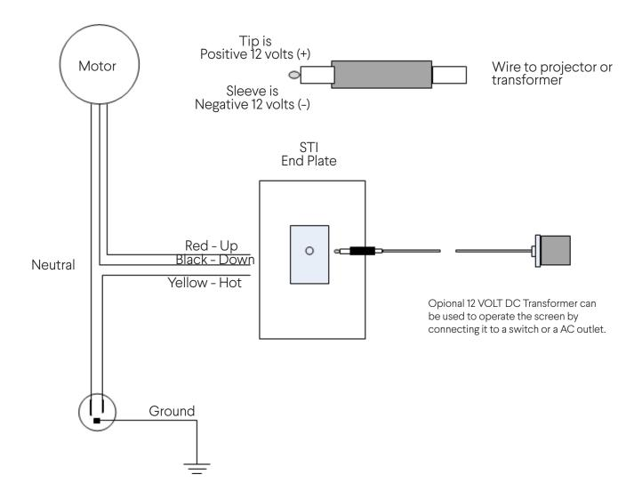
The Stewart Filmscreen Screen Trigger Interface (STI) is a factory-installed control interface that has been designed specifically for the Stewart ElectriScreen motors. A constant 5 – 12 VDC trigger signal activates the STI to lower the screen. Termination of this signal will prompt the STI to retract the screen. The Stewart STI has been designed to function effectively with all the various trigger outputs from a multitude of projector types.
