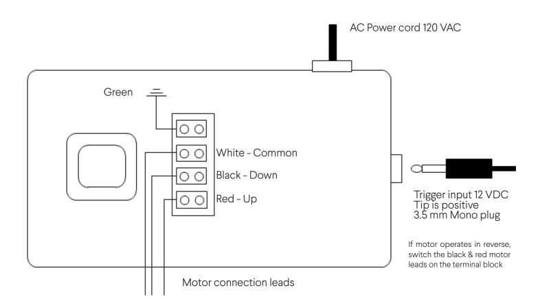
The VICS is an external version of the Screen Trigger Interface (STI). It interfaces with the triggering outputs from projectors, receivers, or other 3rd party control systems.
