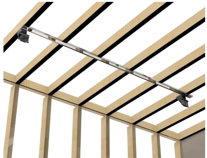
Figure 14. Ceiling brackets screwed onto ceiling joists
