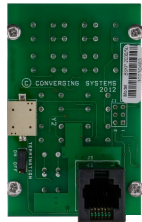
Figure 22. Rear of IR wall switch with RJ25 input
