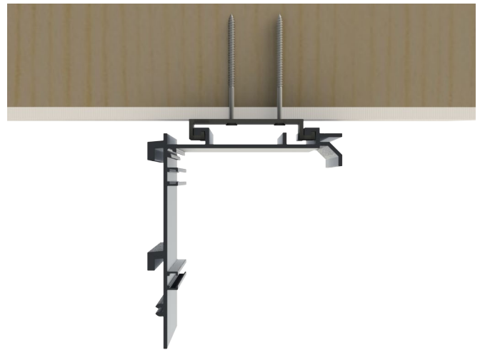
Figure 9. Ceiling bracket screwed onto ceiling joists
