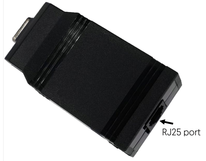
Figure 25. IBT-100, showing RJ25 port
