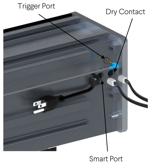
Figure 18. Rear, audience left of case with 10 ft power wire, two RJ45 inputs and a 3.5 mm trigger port
