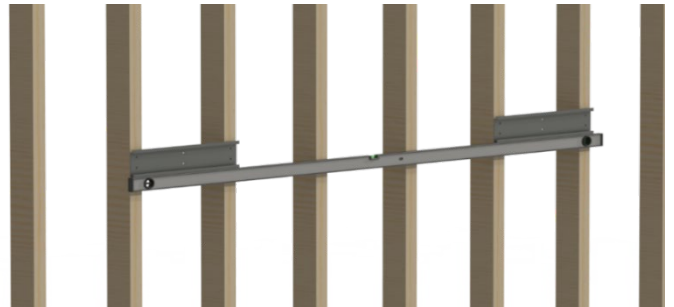
Figure 5. Wall mounts leveled and attached to one or more wall studs
