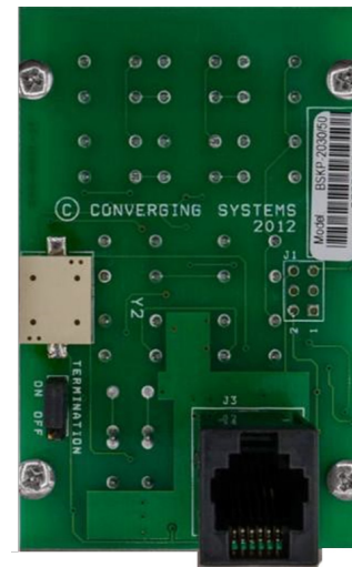
Figure 14. Rear of wall switch with RJ25 input
