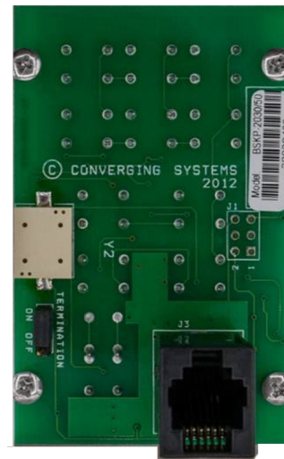
Figure 20. Rear of wall switch with RJ25 input
