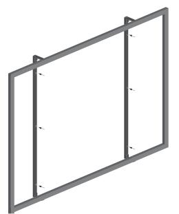
Figure 7: Positioning the Frame and Wall Boards to the Wall
