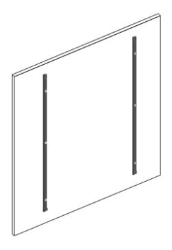
Figure 12: Pocket Mounts on Wall
