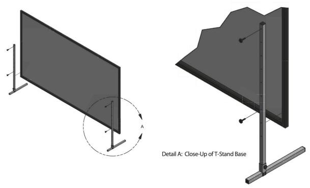
Figure 11: Attaching T-Stand Knobs
