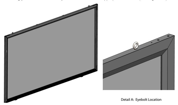
Figure 10: Eye Bolts Mounted Securely to the Frame
