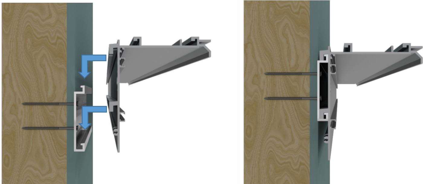
Figure 7: Cross-sectional renders above, showcase the ease of installing the wall mount bracket to the Luxus G2 railing system.
