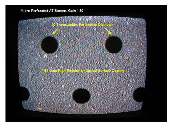
Please note that the perforated sample, at the same magnification, has only 5 significant voids, which is exactly 10.2% of the surface area, and has minimal effect on the picture.
