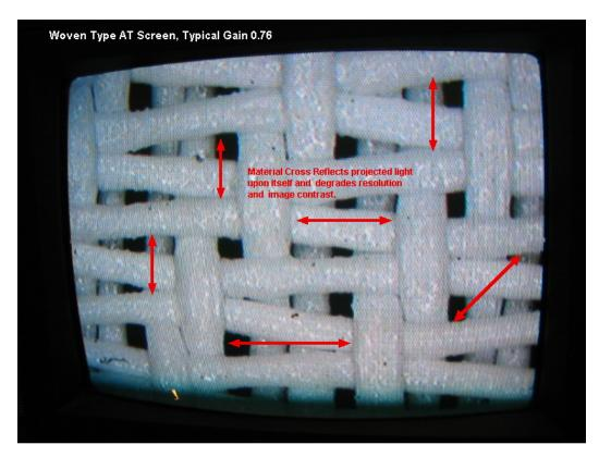
Since we previously measured that there is light "blow through", one can clearly see that this is due to the 20 significant voids and countless undulated "yarn" surfaces which distribute light in an indiscriminate manner.
